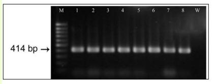
Tumorigenic (Ti) plasmid was detected in all strains by PCR using primers designed to amplify the virC pathogenicity gene, producing a 414-bp PCR product.
