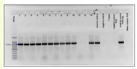
Agarose gel showing Xap specific band at 800 bp (Audy *et al.*,1994 primers).
