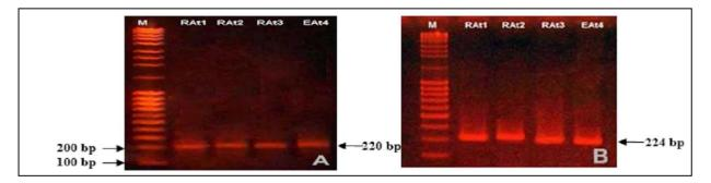
Amplified products resulted from the use of the two specific primers: tms2A/tms2B, (A); virD2A/virD2C (B); M: a 100 bp DNA marker ladder.
