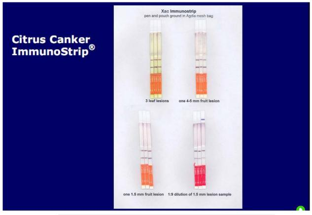
Positive samples produce two colored bands; Negative samples produce a single control band.
