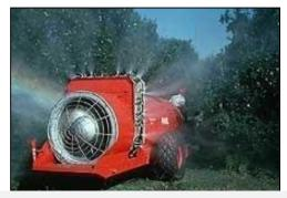
Typical airblast sprayer in citrus planting used to apply agrochemicals such as copper for control of citrus canker.
