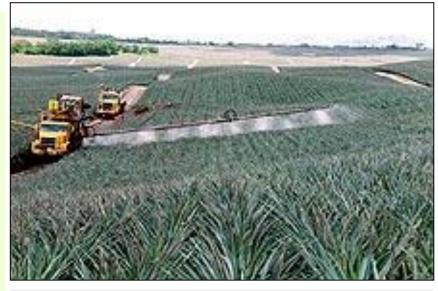
Application of insecticide by means a long arm boom sprayer extending both sides of supplier truck.
